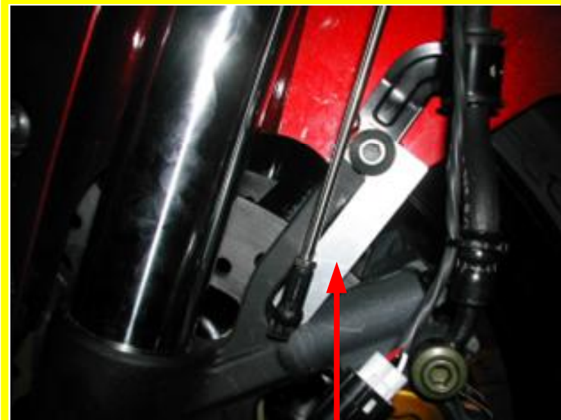
Special mounting kit to fix the lower part of the front suspension sensor
